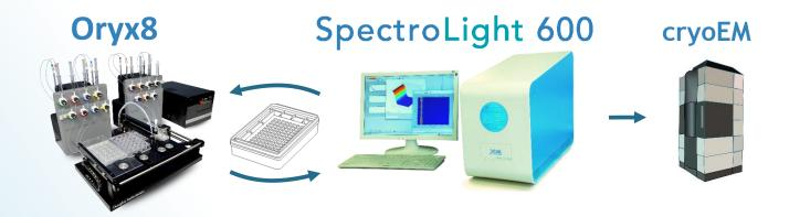
Screening and optimization experiments (with cryoEM and/or crystallography in mind) can be dispensed by the Oryx8, then efficiently analyzed by the SpectroLight 600.
